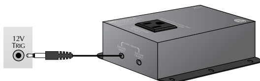
Figure 6 - 12-Volt Trigger Output Connection
